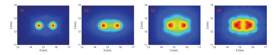
Atomistic tight-binding simulation of the four lowest electronic states of a P2+ donor molecule in Si (shown as 2D cuts).
