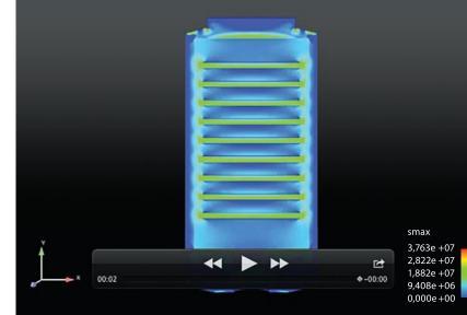
not be well understood. While dynamic stresses from vibration and impact are important, understanding the residual manufacturing stress is a critical first step for determining margins. For this effort, common packaging materials were characterized and nonlinear constitutive models were populated to perform computational simulations. Coupled physics, quasistatic thermal stress, preload, and dynamic impact simulations were utilized to investigate the advantages and disadvantages of various
