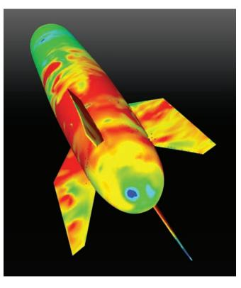
Navier-Stokes/LES method and the response of the structure to this loading is computed using Sandiadeveloped Sierra-SD (structural dynamics) solver.
