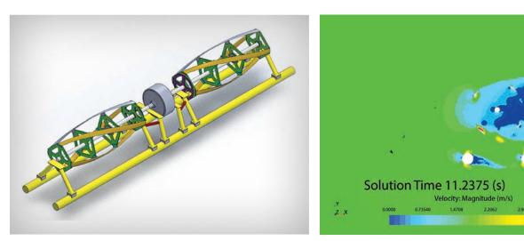
Numerical experiments, simulated on Glory, were then conducted to investigate and quantify parasitic drag effects on turbine performance and how these effects could be mitigated to improve performance. The results of this investigation provided a clear path for modifications to be made in the next design iteration of the RivGen turbine.
